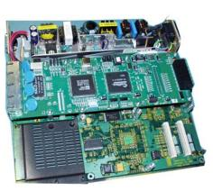
after successfully installing the 6KPM cards inside the Magnum 6K16-Series.
